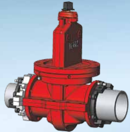
Install new downstream pipe.
