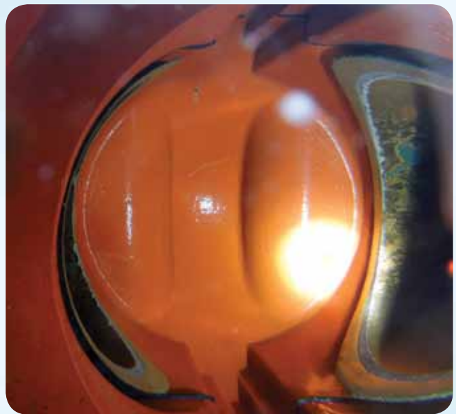
Internal view of the actual InsertValve under 100 psi working pressure.
